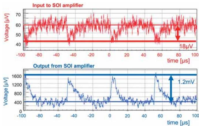
**Fig. 3.** The signal from Nb/AI-STJ to the SOI amplifier (upper) and the amplified output (lower).
