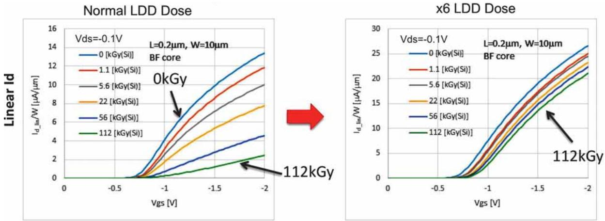
**Fig. 2.** Drain current decrease by irradiation. (Left) normal LDD dose case. (Right) six times higher LDD dose case. The effect of the irradiation is very much reduced.
