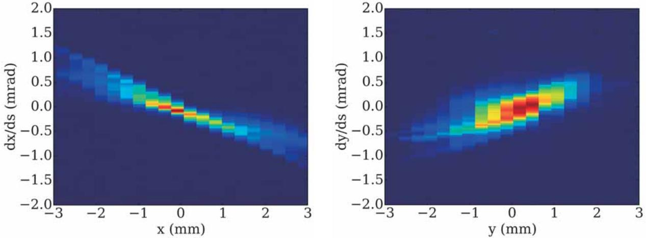
**Fig. 1.** Emittance measurement experimental data at the condition of 40 pC/bunch by using slit scanning method on (a) horizontal direction and (b) vertical direction, respectively.
