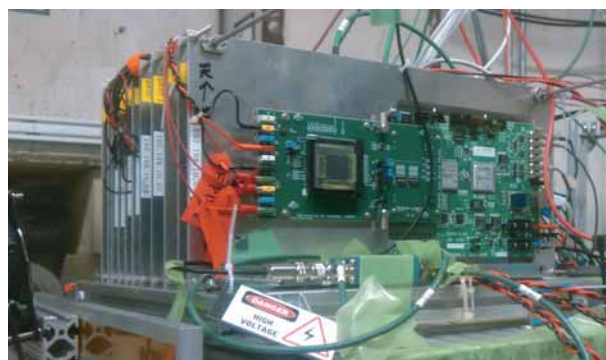
Fig. 2. SOIPIX sensor stack involving four FPIX2 and two SOFIST1 sensors used for the beam test in Fermilab.
