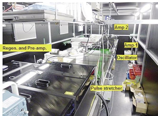
Fig. 5. The 10 TW Ti: Sapphire laser for LWFA.
