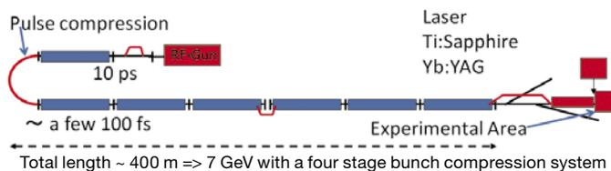
Fig. 4. Facility concept of Ultra High Intensity Beam-Laser Complex using the existing KEK LINAC.
