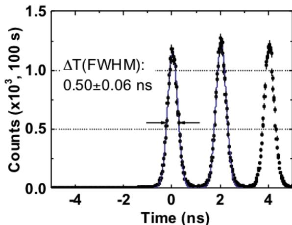
Fig. 3. Pulse train of X-rays, recorded in the PF beam line by the demonstration prototype for FSCI.
