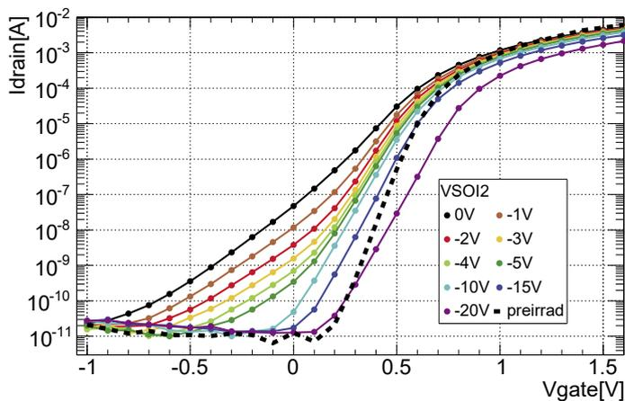
**Fig. 1.** I-V curves of the SOI test FET. The dotted curve represents the I-V behavior before irradiation. After a 2000 kGy exposure to radiation, the curve shifts to the black line. Application of a compensating voltage ( $V_{SOI}$ ) brings the curve gradually back and finally to the purple line at 20 V close to the pre-irradiated level.
