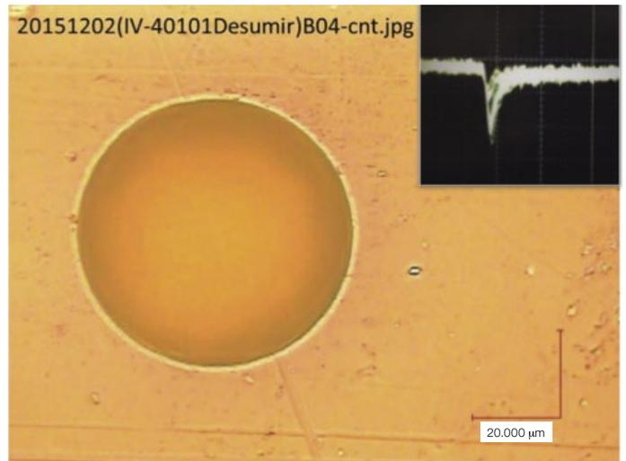
**Fig. 2.** Microscope image of the new GEM film. The laser-etched hole of 70  $\mu\text{m}$  is clearly visible. Inset shows an oscilloscope trace observed for 5.9 keV X-rays.
