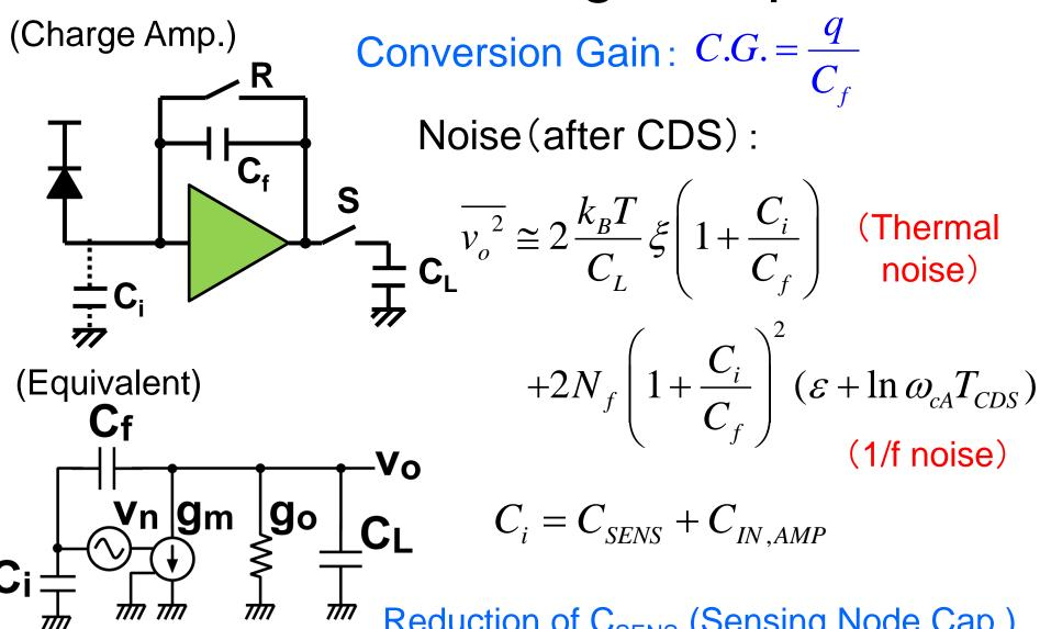
Reduction of  $C_{SENS}$  (Sensing Node Cap.) and  $C_{IN.AMP}$  (Amp. Input Cap.) is important.
