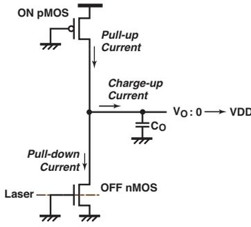
Fig. 8. Equivalent circuit model for waveform analysis.
