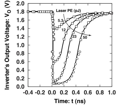
Fig. 10. DSET waveforms obtained when the target inverter was irradiated with various laser PEs.
