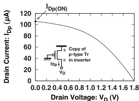
Fig. 12.  $I_D$  versus  $V_D$  curve for the  $p$ -type transistor in the target inverter. We fabricated a copy of the  $p$ -type transistor M1 and measured its drain currents as a function of the drain voltage.
