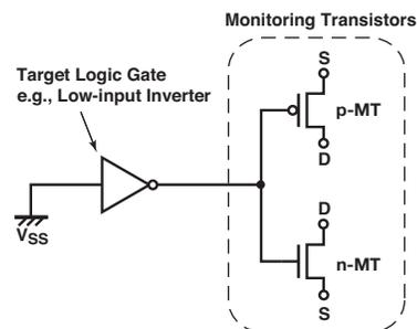
Fig. 1. Proposed circuitry. The output of a target logic gate is connected to the gate inputs of two elementary MOS transistors, one of which is an  $n$ -type transistor and the other of which is  $p$ -type. The connected transistors named “monitoring transistors (MTs)” fulfill the roles of a DSET monitor.
