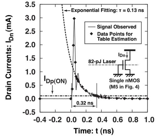
Fig. 9. Transient drain current induced by laser irradiation in the single  $n$ -type transistor (M5). The transistor was in an off-state when its gate was grounded and the drain was biased at a power supply voltage  $V_{DD}$  of 1.8 V. The laser pulse energy (PE) was 82 pJ. The on-current in the  $p$ -type transistor  $I_{Dp(ON)}$  labeled in Fig. 6 and an exponential fitting line are superimposed. Symbols indicate the data points used in the table-based estimation. See also the appendix.
