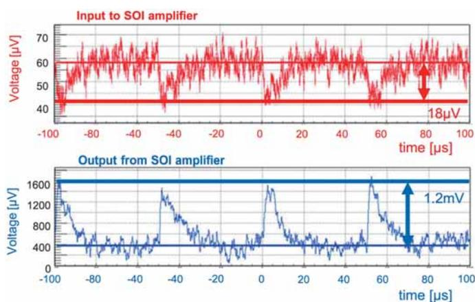
Fig. 3. The signal from Nb/Al-STJ to the SOI amplifier (upper) and the amplified output (lower).
