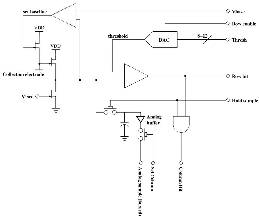
**Figure 4: Essential elements of each pixel cell. A comparator is used to determine the crossing of a threshold set with an in-pixel DAC. A feedback loop is used to compensate for leakage current and restore the baseline after collection of an induced signal.**
