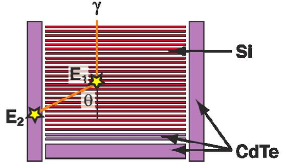
Figure 1: The Imaging Hard X-ray Compton Polarimeter (IHXCP) concept.
