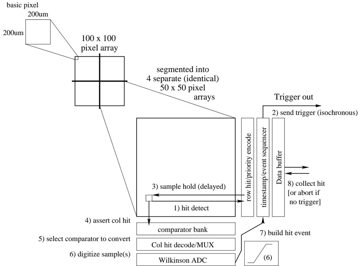
**Figure 3: Overview of the readout architecture, illustrating the data-driven nature of the proposed scheme. A hit is encoded and collected as per the enumerated steps shown and described in more detail in the text.**
