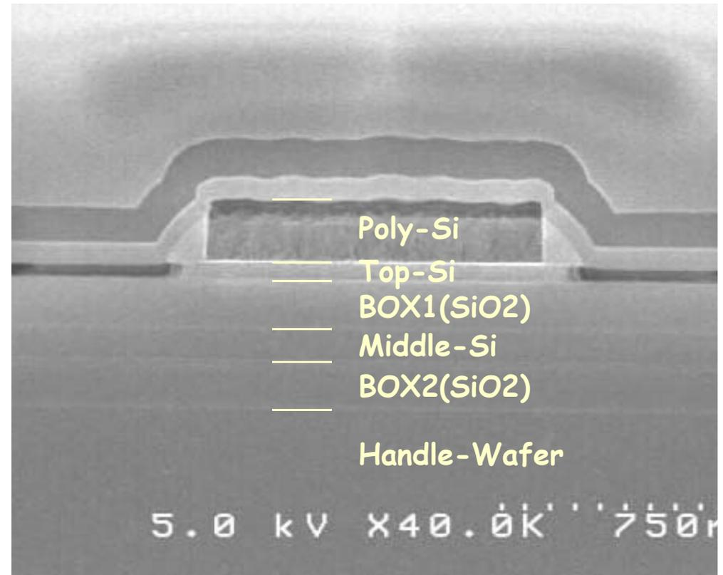
(Thickness of Si & SiO<sub>2</sub> layers are not yet optimized)
