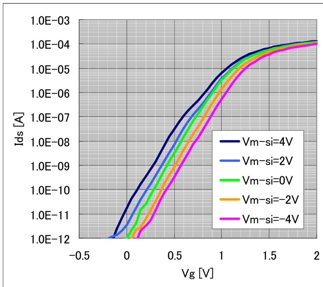
Threshold voltage of a transistor is controlled with the bias voltage of the Middle-Si layer. This indicates effects of the trapped charge in the BOX can be compensated with the bias voltage.
