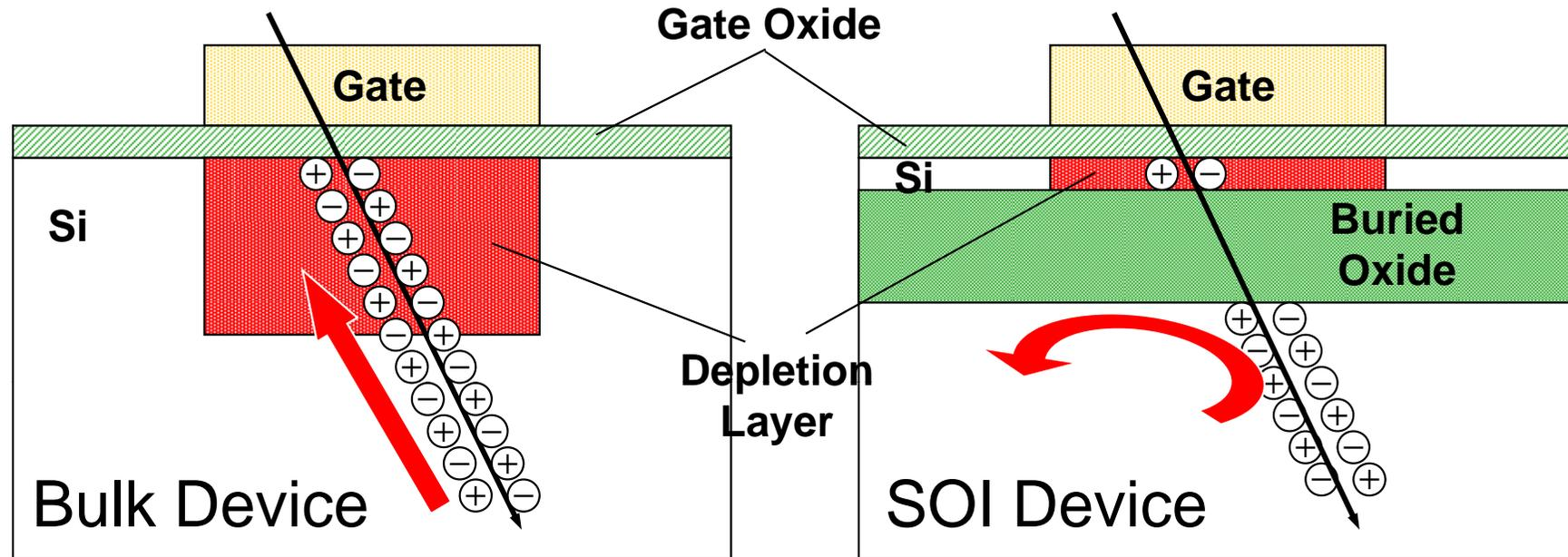
But not necessary strong to Total Ionization Dose due to thick BOX layer
