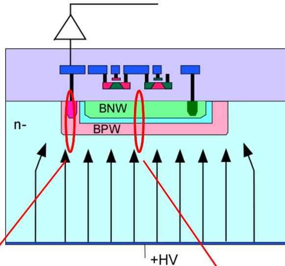
Peaks of BNW and BPW are separated  $\sim 0.7 \mu\text{m}$  to reduce capacitance
