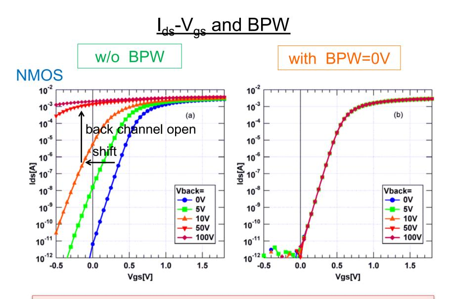
Back-gate effect is completely suppressed by the BPW.
