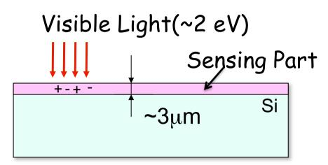
Visible Light ~ 1 e-h / 1 photon High Energy Particle ~ 80 e-h / μm X-ray ~ 3000 e-h @10 keV
