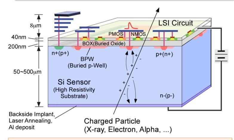
Monolithic Detector having fine resolution of silicon process and high functionality of CMOS LSI by using a SOI Pixel Technology.
