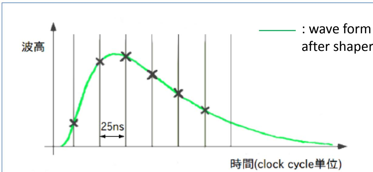
APV25 chip has a function of data sampling
