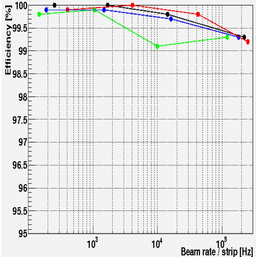
If the beam spot size is a few cm ( $\phi$ ) , SSD can work under 10 MHz .
