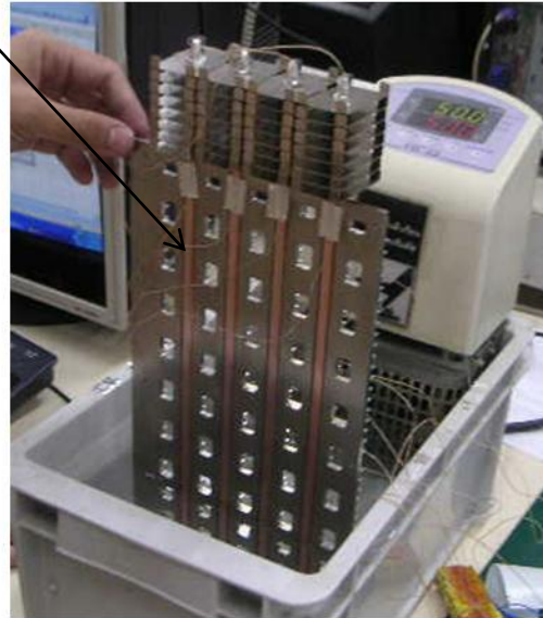
Heat Pipe Cooling Module Sample
