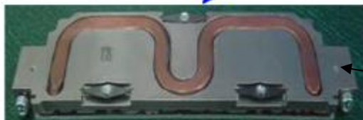
Heat spreader Plate(DMS1) with Heat pipe
