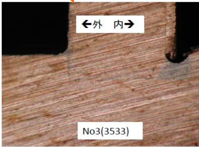
Brazed Cold Plate (Cross Section)
