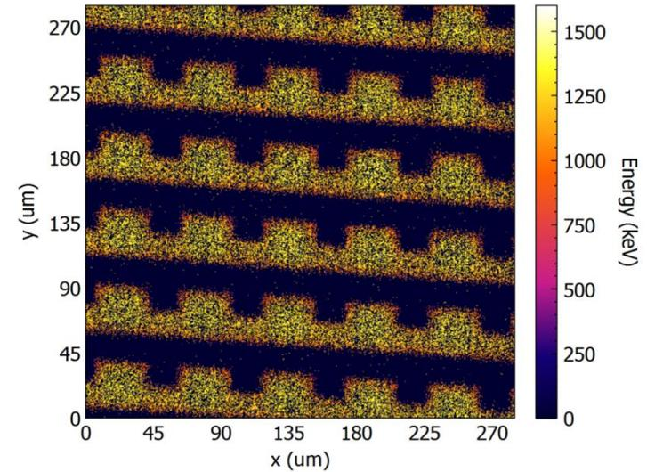
Energy spectrum and median energy map showing the spatial distribution of energy deposited by 5.5 MeV He<sup>+</sup> ions in the SVs of the odd and even arrays. The detector was at -10 V
