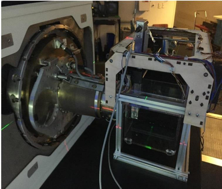
Left: Moveable water phantom with Bridge Microdosimeter in front of PBS nozzle.
