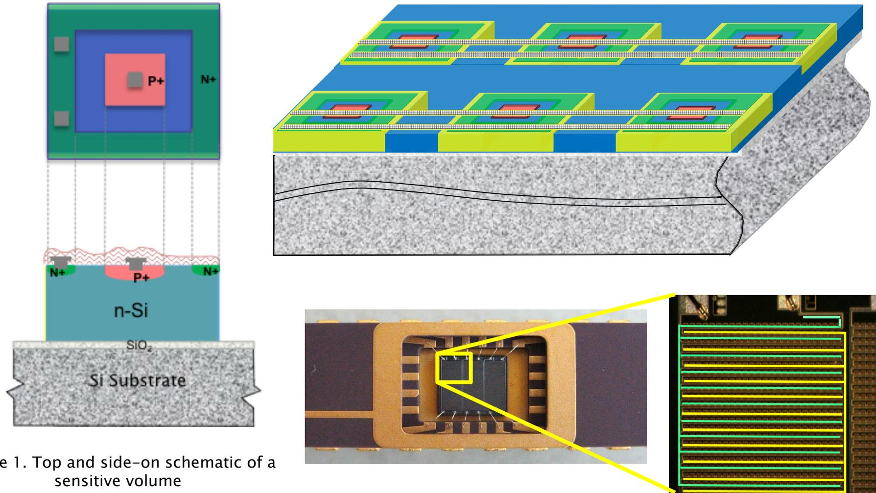
Figure 1. Top and side-on schematic of a sensitive volume
