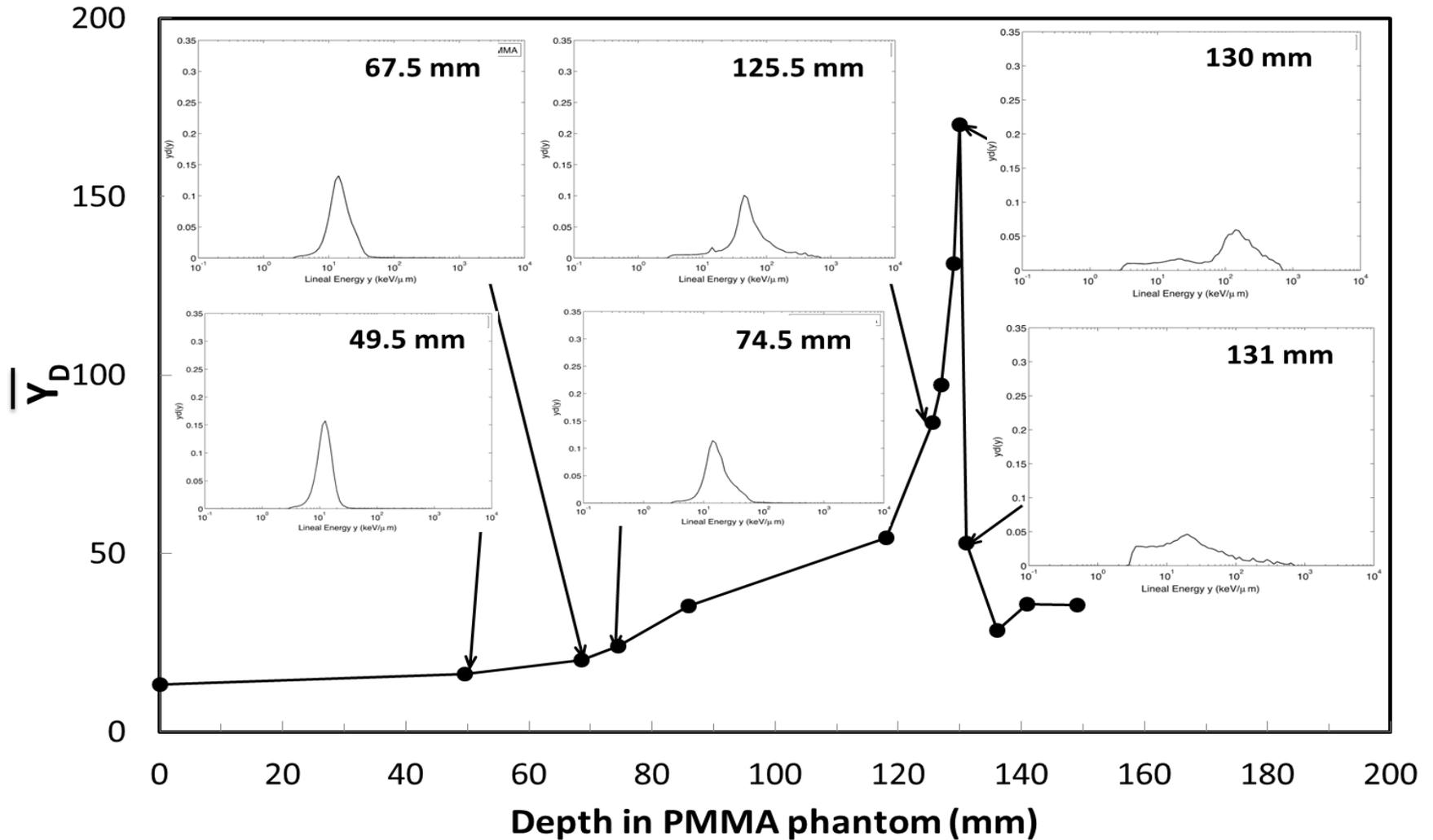
Dose-mean lineal energy deposition and microdosimetric spectra obtained along the SOBP
