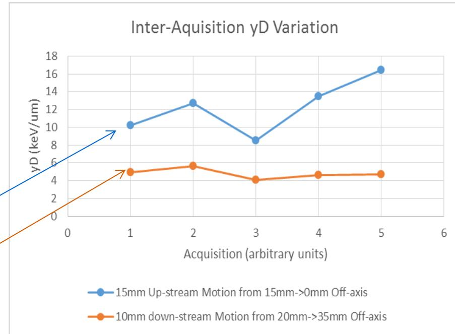
$y_D$  when moving and stationary, 10mm Down Stream and 15mm Up Stream from isocentre
